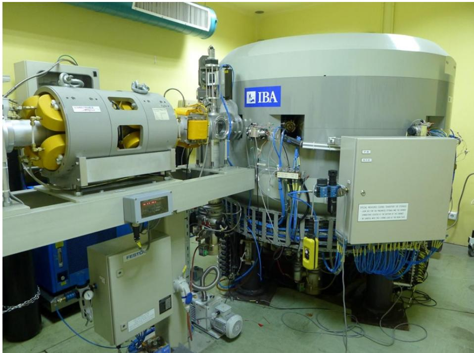
Figura 2.6: Ciclotrón 18/9 MeV del CNA / Cyclotron 18/9 MeV at CNA
